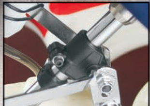
ARROW'S UNIQUE STEERING BUSH WITH CLAMP FOR SIMPLE FRONT WHEEL ALIGNMENT
