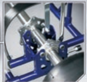
40mm axle supported by machined billet alloy bearing carriers
