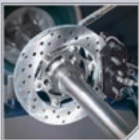
Machined billet alloy 2-spot brake caliper anodised black
