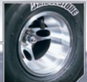
Arrow silver/black one-piece machined alloy 3-spoke wheels
